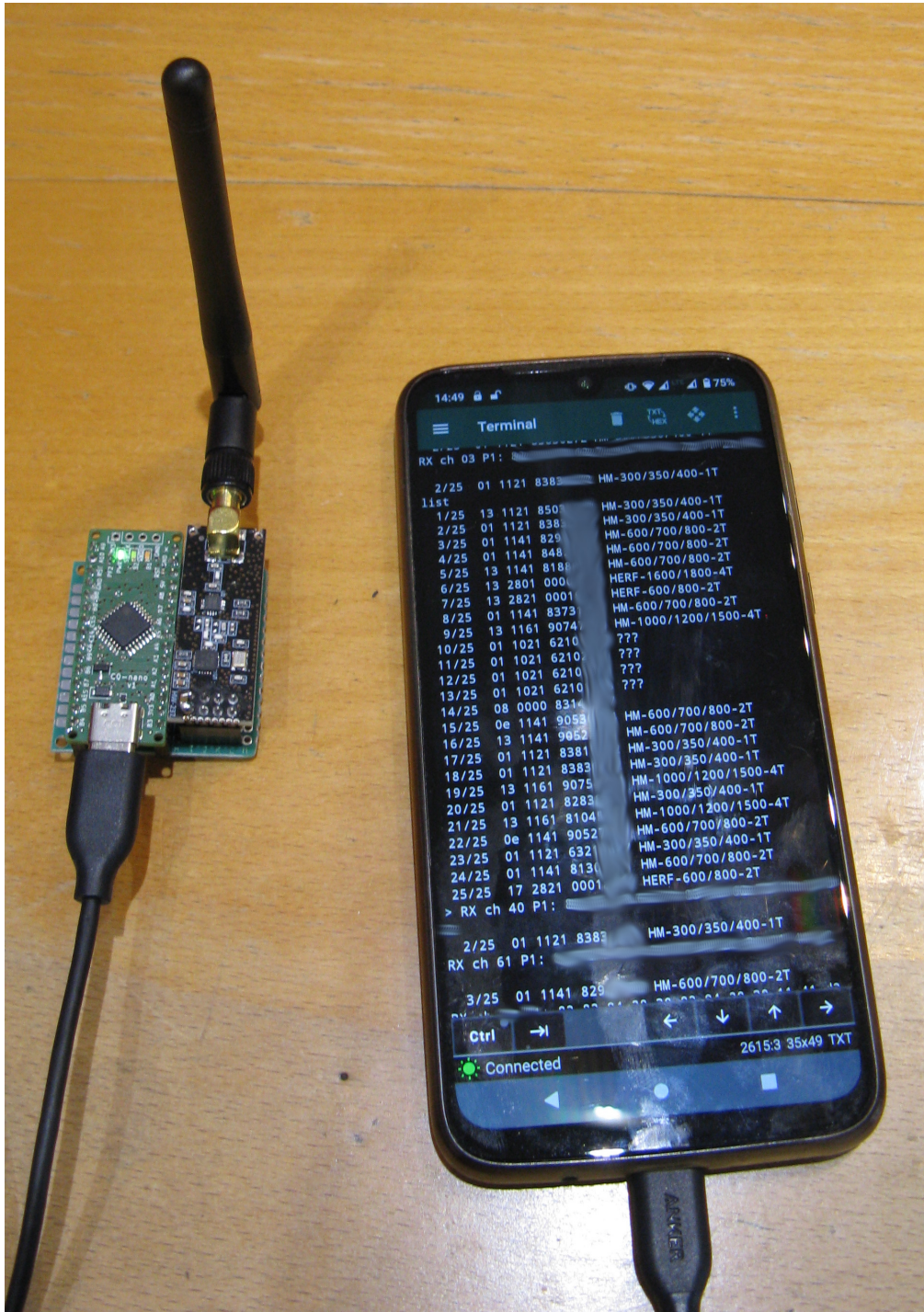
Figure 5: HM series inverter scanner proof-of-concept
